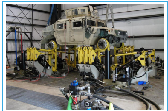
Figure 1. Up-armored HMMWV testing on the ATC VDS(Vehicle Durability Simulator)
