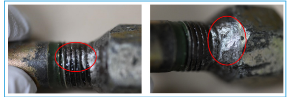
Figure 7. Damaged traces of bolt screw thread(left) and base side of nut(right)
